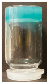
Fig. 2 Metallogel formed from the reaction of \text{L}^1 with one equivalent of copper(II) chloride in \text{H}_2\text{O}/\text{thf} (3 : 2) at 1 wt%.
