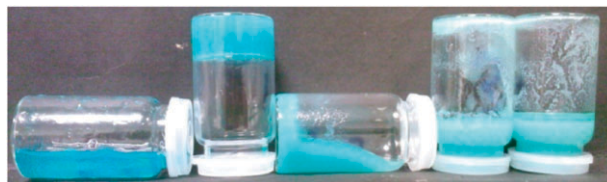
Fig. 3 Copper(II) chloride gels formed with \text{L}^1 in varying ratios; left to right, copper(II) chloride : \text{L}^1 ratios 0.5 : 1, 1 : 1, 2 : 1, 4 : 1 and 8 : 1.
